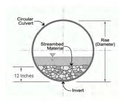
In all other areas: Culverts greater than 48 inches in diameter will be buried at least one foot below the bed of the stream. Culverts 48 inches in diameter or less shall be buried to maintain aquatic passage and to maintain passage during drought or low flow conditions, and every effort shall be made to maintain the existing channel slope.
